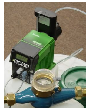
Proportional Dosing System
